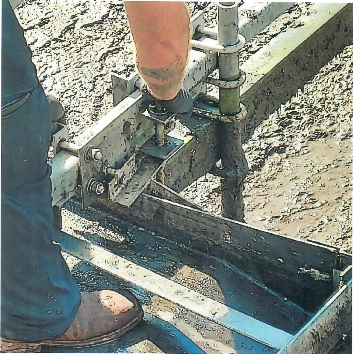
Adjusting the scum arm to reduce torque load
