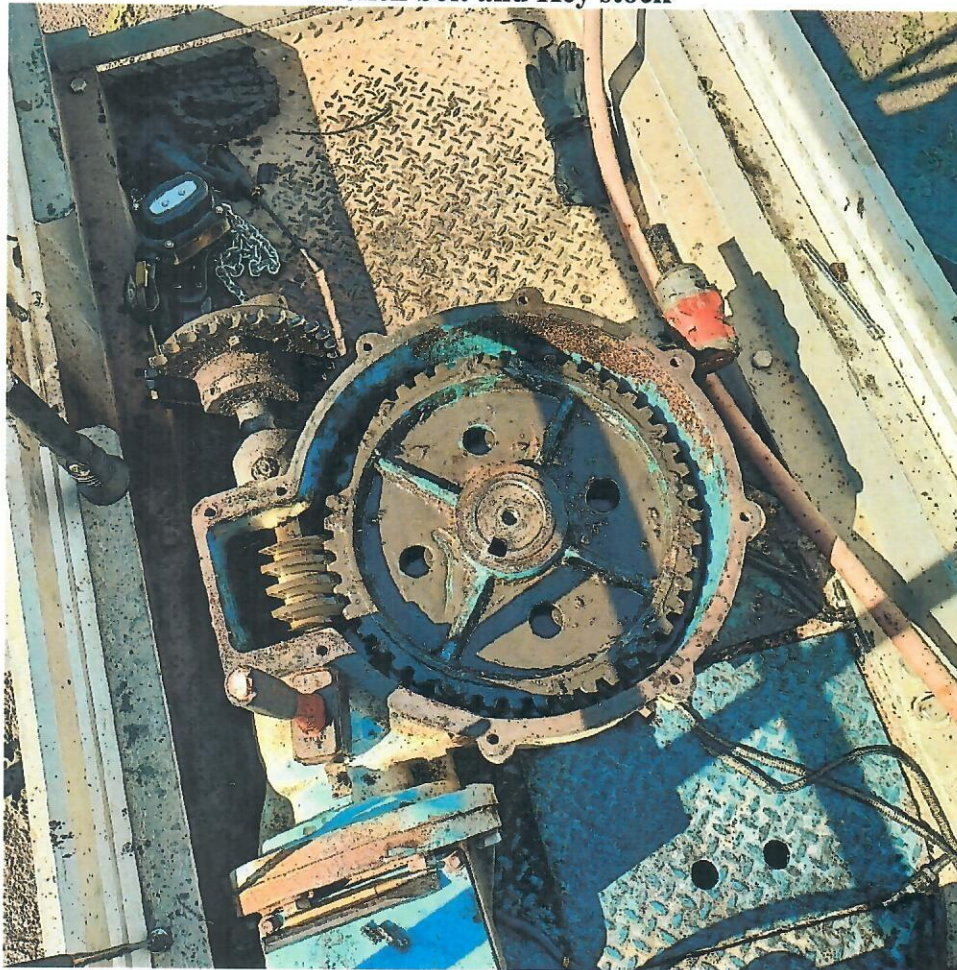
Broken bolt and Key stock
