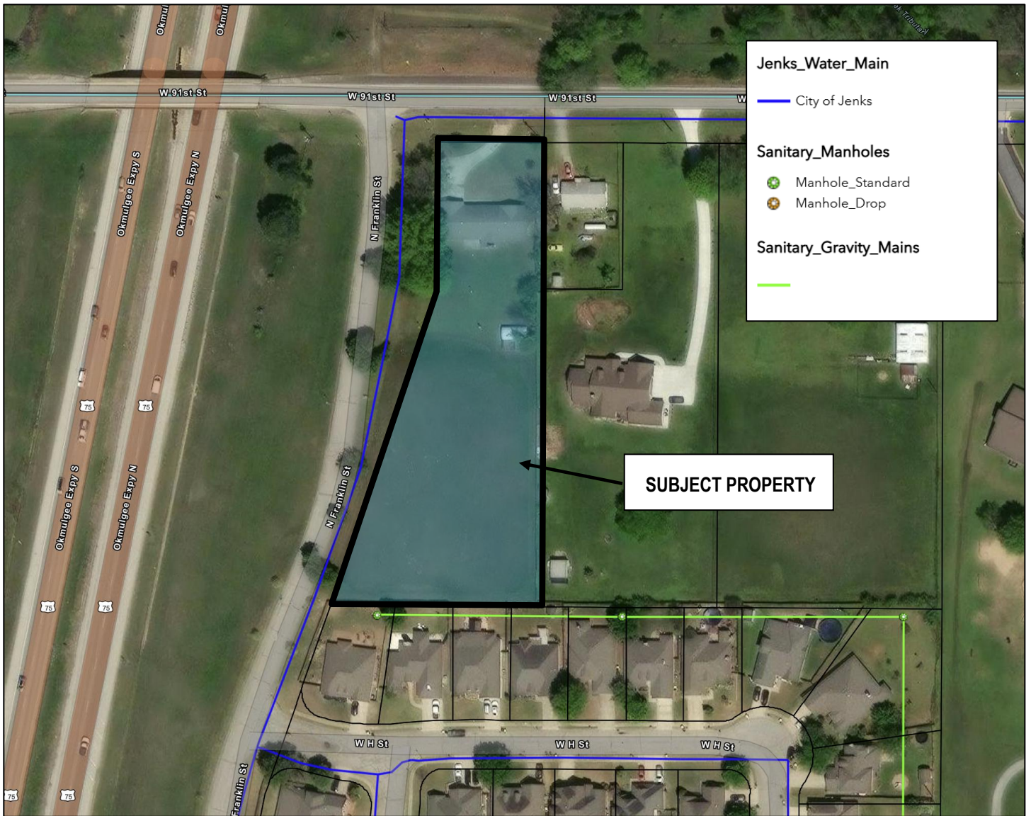
Figure 2: Aerial Map with Water and Sewer Lines
